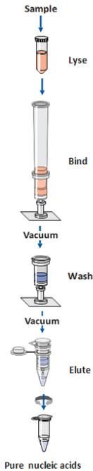
**Figure 1: Procedure of column-based manual, cell-free DNA extraction.**
