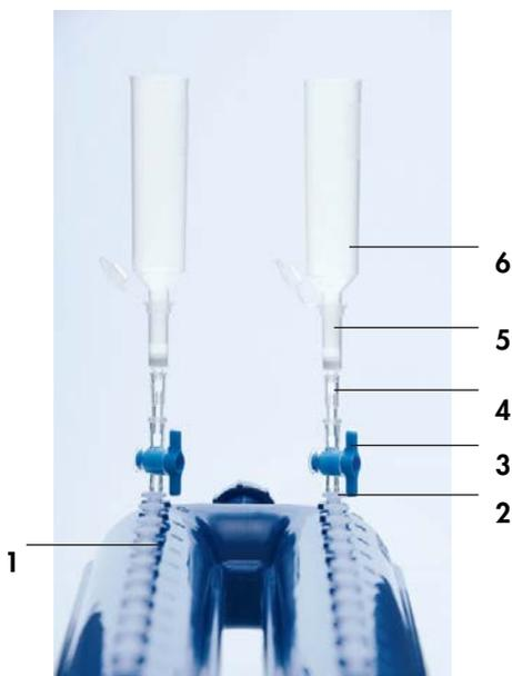
**Figure 4: Setting up the QIAvac 24 Plus with QIAamp Mini columns using VacValves, VacConnectors and Tube Extenders. (1: QIAvac 24 Plus vacuum manifold, 2: Luer slot of the QIAvac 24 Plus (closed with luer plug), 3: QIAamp Mini column, 4: VacConnector, VacValve (must be purchased separately), 6: Tube Extender).**
