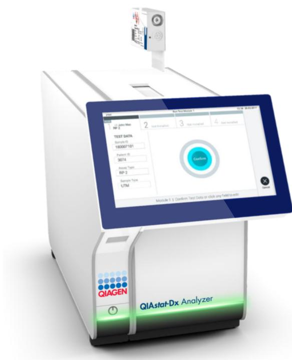
**Figura 28.** Inserindo o QIAstat-Dx Respiratory SARS-CoV-2 Panel Cartridge no QIAstat-Dx Analyzer 1.0.
