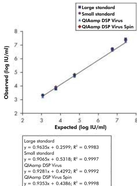
**Figure 2. The linear range of the QIAamp DSP Virus Spin Kit.** The linear range of yields using the QIAamp DSP Virus Spin Kit (cat. no. 61704) with 1 manual and 2 different automated protocols, compared to the manual QIAamp DSP Virus Kit (cat. no. 60704) procedure using the QIAvac 24 Plus. The linear range of the protocols was determined using viral dilution series and an in-house RT-PCR assay for HCV RNA.
