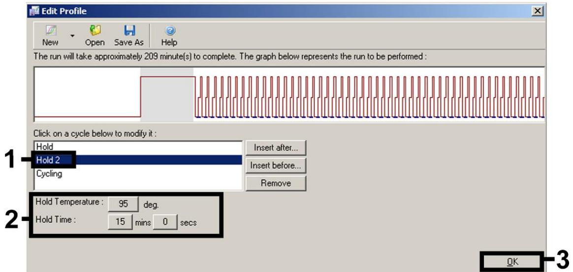
**Figure 9. Initial activation of the hot-start enzyme.**
