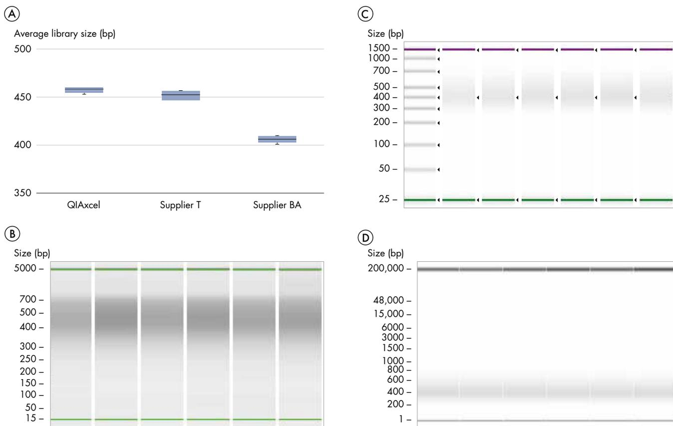
**Figure 1. Comparison of reproducibility between the microfluidic electrophoresis platforms.** Average fragment size (bp) was determined using a single Illumina DNA Prep (M) Tagmentation library, performed in technical replicates (n=6). **A:** Box and whisker plot showing the comparison of average fragment sizes (bp) between the QIAxcel Advanced, Supplier T and Supplier BA. **B:** QIAxcel gel image. **C:** Supplier T gel image. **D:** Supplier BA gel image.
