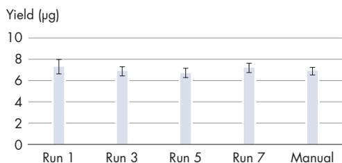
**Figure 1. High yields of RNA.** RNA was isolated from Jurkat cells using the RNeasy Mini Kit. Preps were automated on the QIAcube (runs 1, 3, 5, and 7) and also performed manually. RNA was quantified by measuring the optical density. High yields were obtained for both automated and manual procedures.
