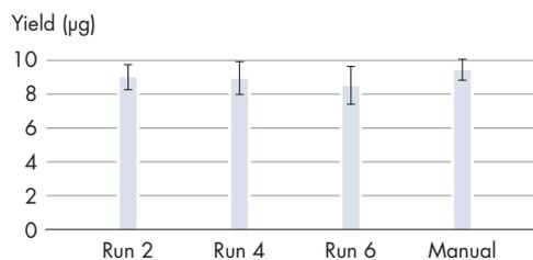
**Figure 4. High yields of plasmid DNA.** pCMV $\beta$  plasmid DNA was purified manually and on the QIAcube. Optical density measurements showed consistently high yields for both methods.
