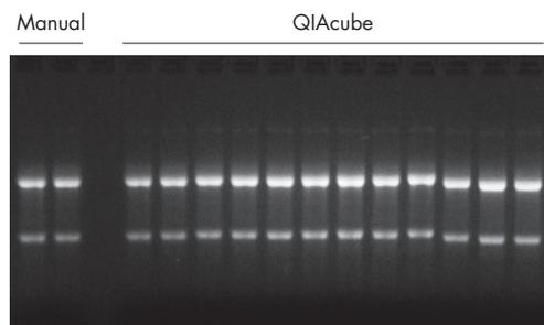
**Figure 2. Analysis of RNA by gel electrophoresis.** RNA preps were performed using the RNeasy Mini Kit, either manually or automated on the QIAcube. RNA was run on a 1.2% agarose gel in Buffer FA (120 V for 90 minutes). The same amount of each sample was used for agarose gel analysis. The integrity of the RNA was preserved after both manual and automated processing, as can be seen from the agarose gel.
