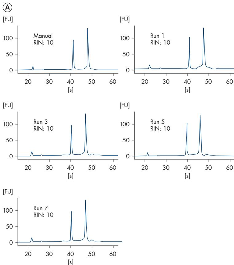
**Figure 3. High-quality RNA preps.** Preps were automated on the QIAcube (runs 1, 3, 5, and 7) and also performed manually. RNA was analyzed on the Agilent 2100 Bioanalyzer. **A** RIN numbers demonstrate the high quality of the purified RNA. **B** No fragmentation or degradation was observed.
