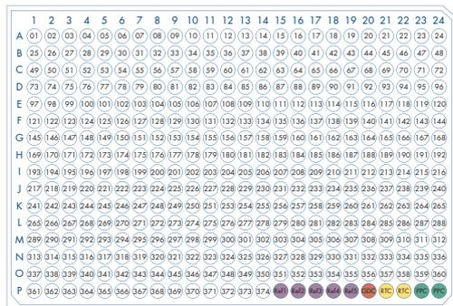
Catalog High-content RT<sup>2</sup> PCR Array plate layout for 384-well qPCR instruments.
