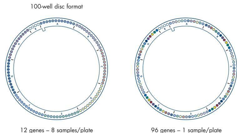
Figure 12. The layouts of the Custom RT<sup>2</sup> PCR Array Ring.
