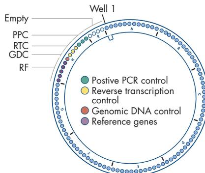
Catalog RT<sup>2</sup> PCR Array plate layout for 100-well rotary qPCR instruments.
