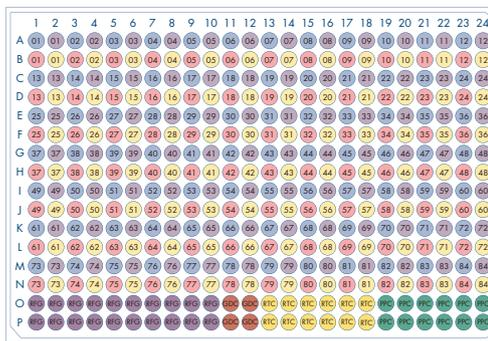
Catalog RT<sup>2</sup> PCR Array plate layout for 384-well qPCR instruments.
