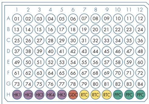
Catalog RT<sup>2</sup> PCR Array plate layout for 96-well qPCR instruments.
