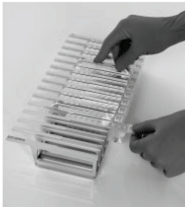
Figure 3. Ease of instrument setup using reagent cartridges. A: A sealed, prefilled reagent cartridge of the EZ1 ccfDNA Mini or Midi Kit. B: Loading reagent cartridges into the cartridge rack. The cartridge rack itself is labeled with an arrow to indicate the direction in which reagent cartridges must be loaded.
