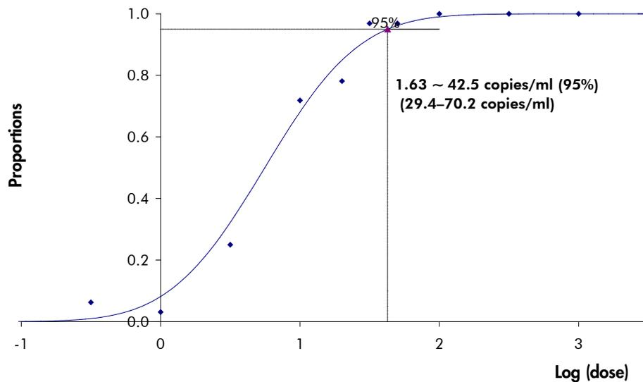
**Figure 1. Probit analysis: plasma, CMV (Rotor-Gene Q).** Limit of detection in consideration of the purification (plasma, using the QIAasymphony DSP Virus/Pathogen Midi Kit) of the *artus* CMV QS-RGQ Kit on the Rotor-Gene Q.
