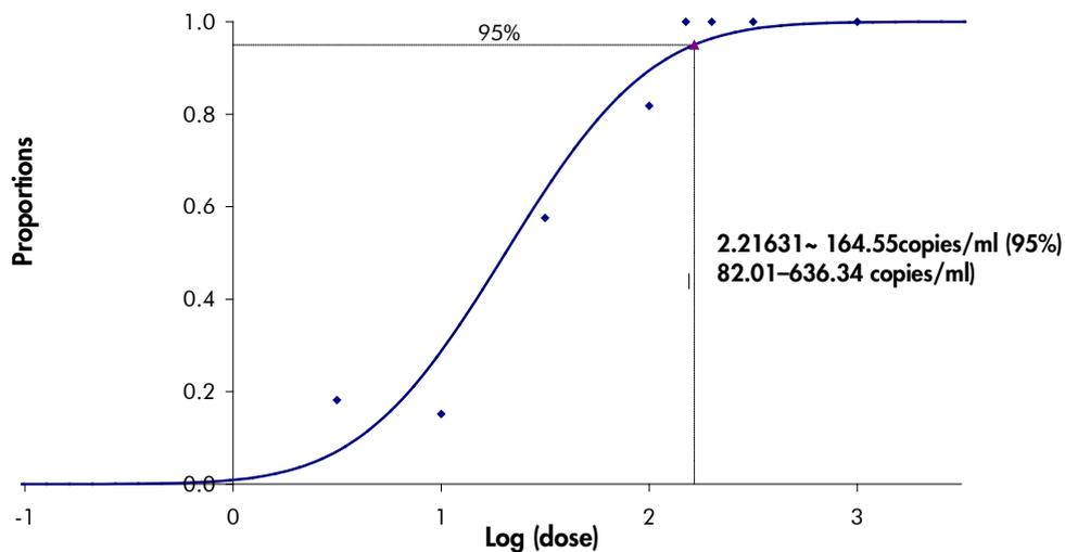
**Figure 5. Probit analysis: whole blood, CMV (Rotor-Gene Q).** Limit of detection in consideration of the purification (whole blood, using the QIA Symphony DNA Mini Kit) of the *artus* CMV QS-RGQ Kit on Rotor-Gene Q.
