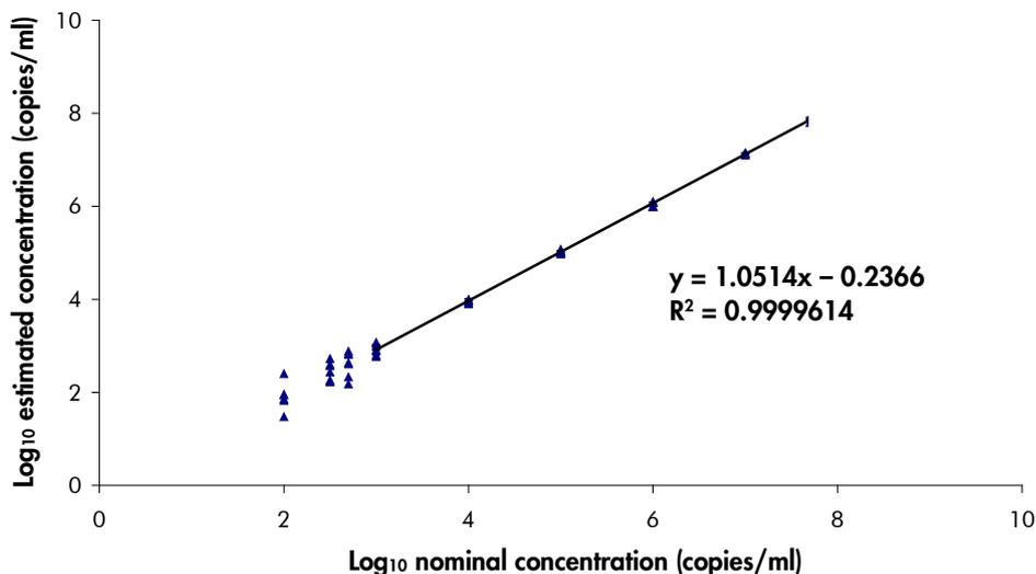
**Figure 6. Linear range of the *artus* CMV QS-RGQ Kit (whole blood).** Calculation of the linear range. The straight line was determined by a linear regression of the log<sub>10</sub> calculated concentrations with the log<sub>10</sub> nominal concentrations. The equation of the regression line is included in the figure.
