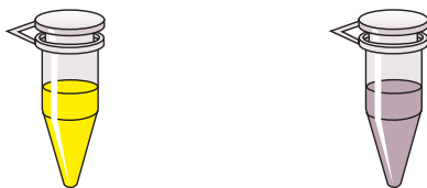
Figure 2. Indicator dye in solubilization and binding Buffer QX1 identifies optimal pH for DNA binding.
