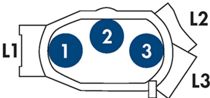
**Figure 7. Positions in the rotor adapter.** The rotor adapter has three tube positions (1–3) and three lid positions (L1–L3).
