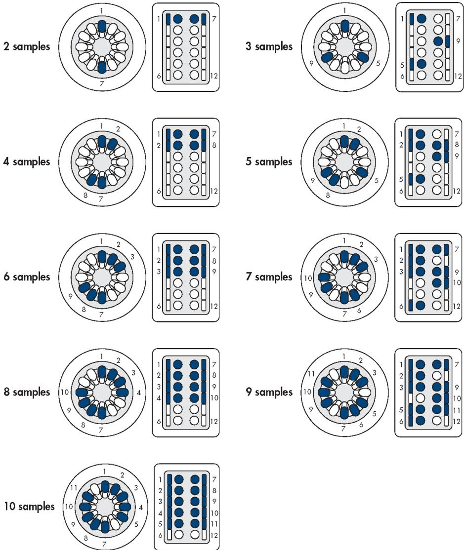
**Figure 9. Loading the centrifuge and shaker.** Centrifuge and shaker positions are shown for processing from two (2 samples) to ten (10 samples) samples. One or 11 samples cannot be processed.
