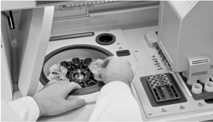
**Figure 8. Loading the centrifuge.** Load the assembled rotor adapters into the centrifuge buckets.
