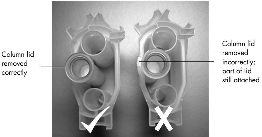
**Figure 6. Loading the PAXgene Shredder spin column.** The PAXgene Shredder spin column is loaded into the middle position of the rotor adapter. Cut off the lid before loading the column.
