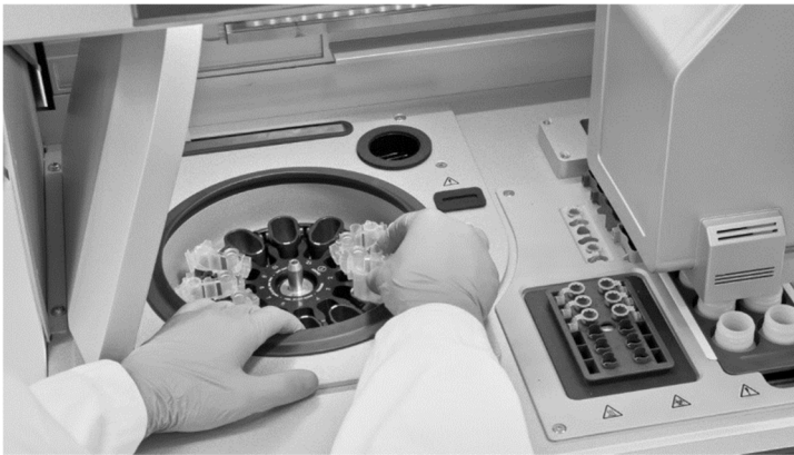
Figure 25. Loading the centrifuge on the QIAcube instruments. Load the assembled rotor adapters into the centrifuge buckets (QIAcube Connect MDx shown as an example).
