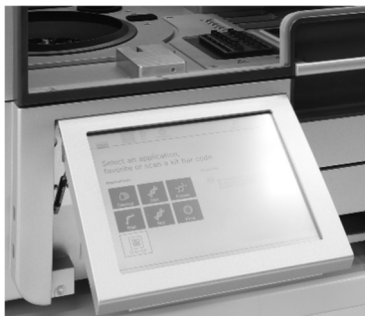
Figure 19. Pulled-out touchscreen of QIAcube Connect MDx
