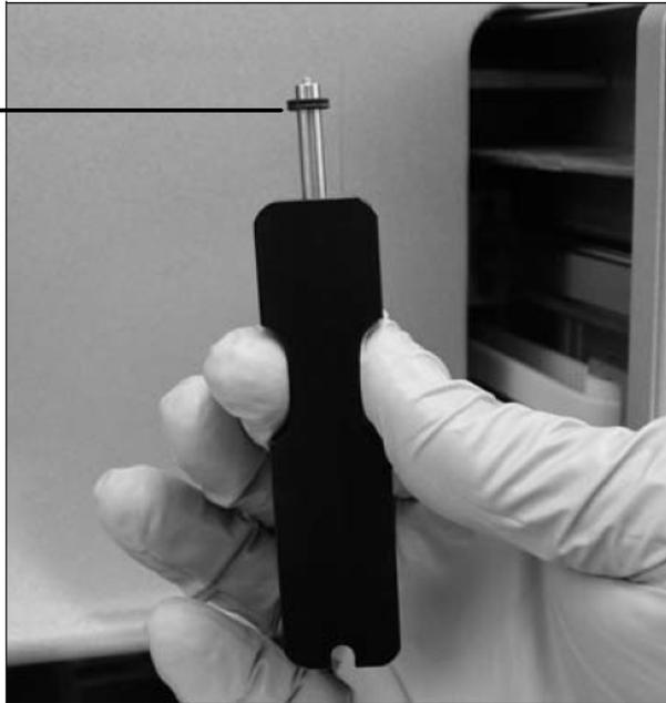
2. Using either your left or right hand, place the ring tool up through the opening for the waste drawer so that the end of the steel shaft is centered in the opening of the tip adapter.
