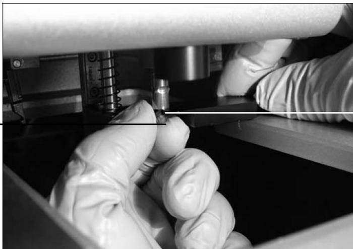
The tool continues to push the tip adapter ring out of its groove
