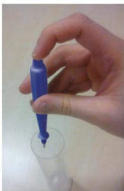
Figure 2. Ejecting the cored sample into the target tube
