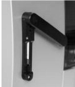
Figure 3. Complete insertion of EZ1 Card. The EZ1 Card must be completely inserted before the EZ1 instrument is switched on.
