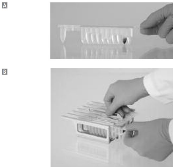
Figure 4. Ease of worktable setup using reagent cartridges. (A) A sealed, prefilled reagent cartridge. Fill levels vary, depending on the type of reagent cartridge. (B) Loading reagent cartridges into the cartridge rack. The cartridge rack itself is labeled with an arrow to indicate the direction in which reagent cartridges must be loaded.
