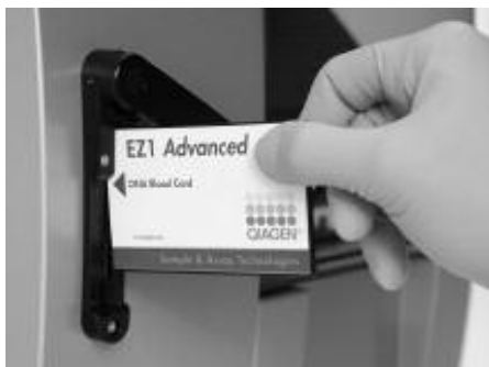
Figure 2. Ease of protocol setup using EZ1 Cards. Inserting an EZ1 Card, containing protocol, into an EZ1 instrument. The instrument should only be switched on after an EZ1 Card is inserted. EZ1 Cards should not be exchanged while the instrument is switched on.
