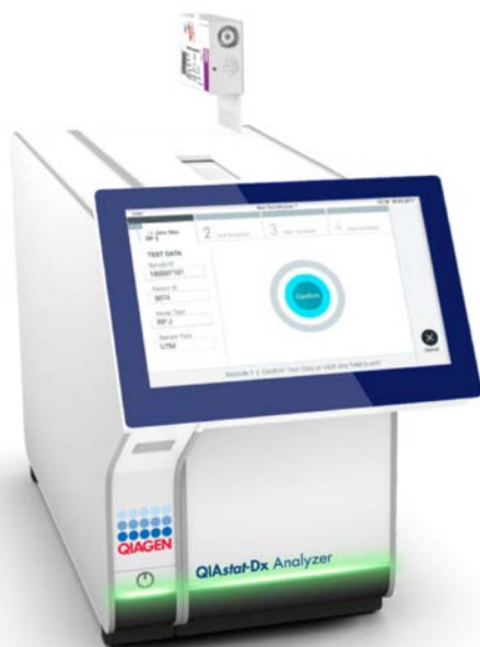
Figura 15. Inserindo o QIAstat-Dx Gastrointestinal Panel Cartridge no QIAstat-Dx Analyzer 1.0.
