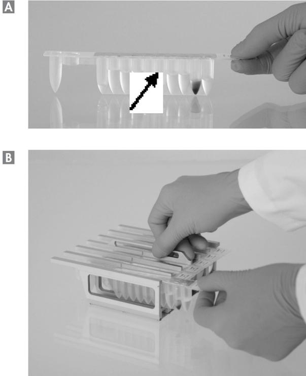
**Figure 3. Ease of setup using reagent cartridges.** (A) A sealed, prefilled reagent cartridge. Fill levels vary, depending on the type of reagent cartridge. Well 5, where DNase I is added by the user, is indicated with an arrow. (B) Loading reagent cartridges into the cartridge rack. The cartridge rack itself is labeled with an arrow to indicate the direction in which reagent cartridges must be loaded.
