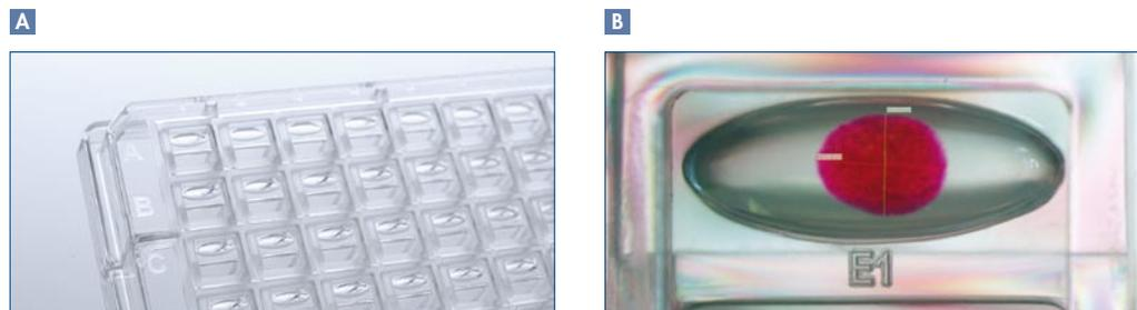
**Figure 13. NeXtal CubicPhase μplate.** **A** Design of precoated NeXtal CubicPhase μplate. **B** Top view of the oval-shaped protein well coated with monoolein (MO). For better visualization, the MO has been colored with a red dye.
