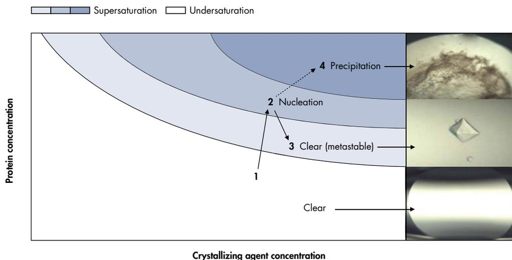
**Figure 4.** The crystallization phase diagram.
