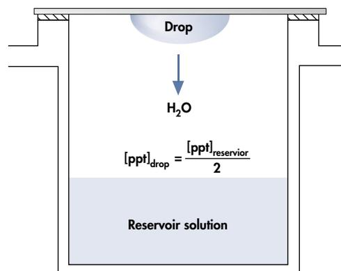
**Figure 3. Principle of a vapor diffusion experiment.**
