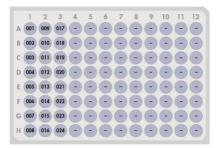
Figure 4. QIAseq UDI Y-Adapter Plate (24) layout (UDI 1-24).
