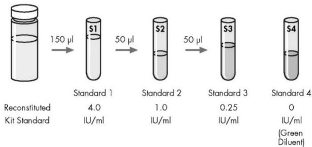
**Figure 2. Preparation of 4-point standard curve**
