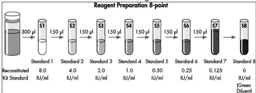
Figure 1. Preparation of 8-point standard curve
