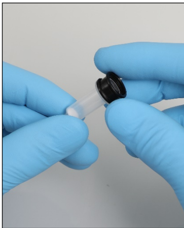
Mounting a spin column adapter ring.
