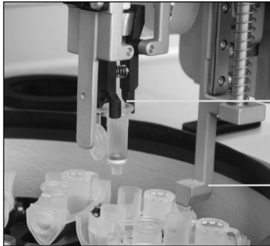
Robotic gripper automates spin-column processing
