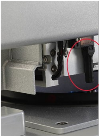
Black beam collimator (see red circle) of the ultrasonic sensor
