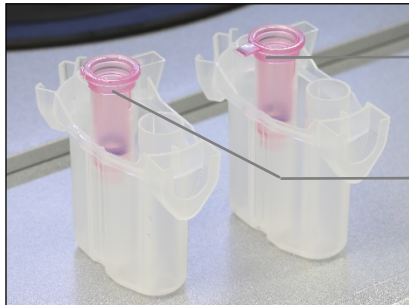
Comparing correct and incorrect removed column lids
