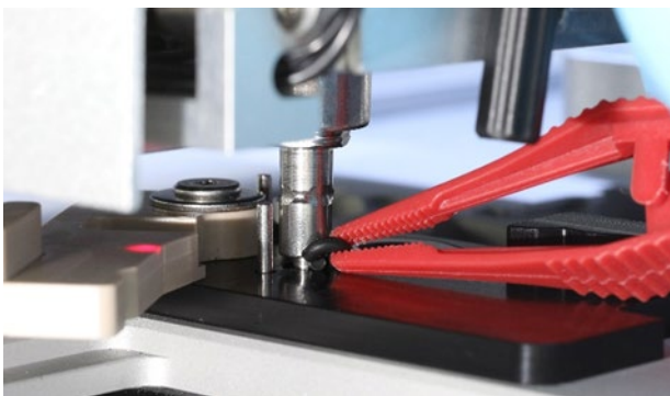
Open the grey lever and remove the O-Ring using the tweezers
