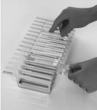
**Figure 4. Ease of setup using reagent cartridges.** (A) A sealed, prefilled reagent cartridge. Fill levels vary, depending on the type of reagent cartridge. (B) Loading reagent cartridges into the cartridge rack. The cartridge rack itself is labeled with an arrow to indicate the direction in which reagent cartridges must be loaded.
