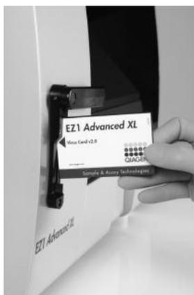
**Figure 2. Ease of protocol setup using EZ1 Cards.** Inserting an EZ1 Card, containing a protocol, into an EZ1 instrument. The instrument should only be switched on after an EZ1 Card is inserted. EZ1 Cards should not be exchanged while the instrument is switched on.
