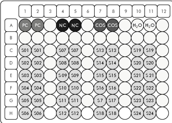
**Figure 3. Suggested plate setup for one experiment with the *ipsogen* MPL W515L/K MutaScreen Kit.** PC: Positive control; NC: Negative control; COS: Cut-off sample; H<sub>2</sub>O: Water control; S: DNA sample.
