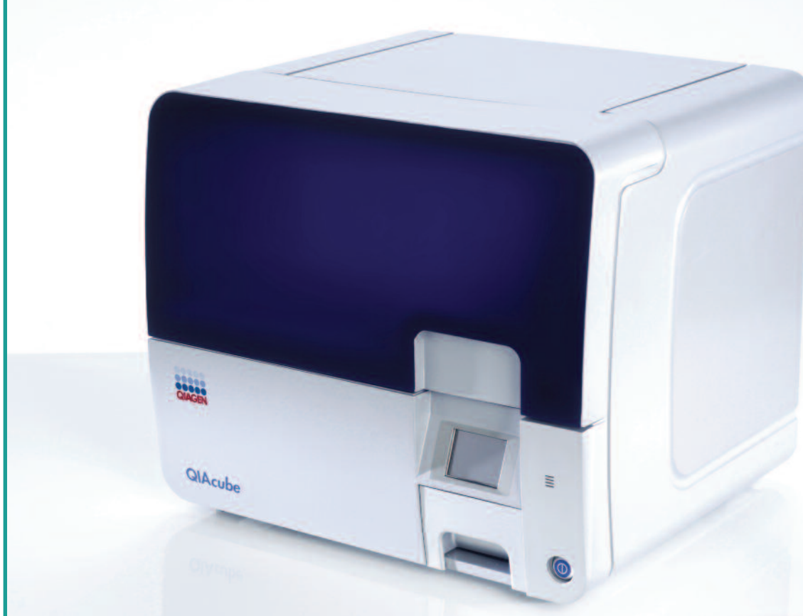
Figure 1. QIAcube® instrument, for automated PAXgene Blood miRNA purification.
