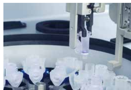
Figure 5. Freedom from laborious manual tasks. The QIAcube is equipped with an automated centrifuge and pipetting system. No manual handling steps are required during the QIAcube run.
