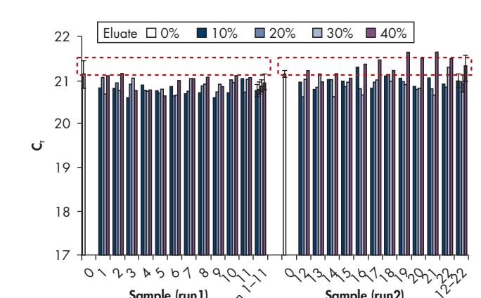
Figure 5 The PAXgene Blood RNA purification procedure was carried out 22 times using distilled water as the starting material instead of the pellet resulting from centrifugation of PAXgene Blood RNA Tubes. Each of the resulting "blank" eluates was used in real-time RT-PCR of the \beta -actin transcript with a constant amount of template RNA. The eluate comprised the indicated percentage of the reaction volume.
