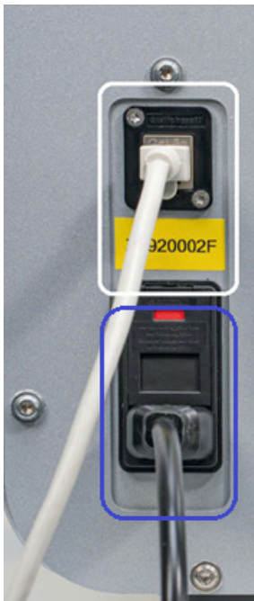
Figure 5. Location of RJ-45 port and power cord socket.
