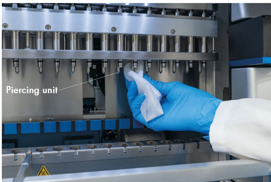
Figure 76. Cleaning the EZ2 piercing unit.
