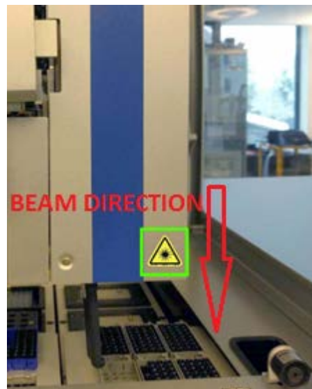
¶ Position 2 for laser light warning label (AS).
