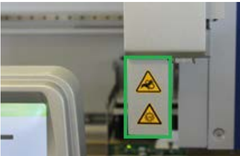
‡ Position of the crushing hazard warning label and UV light warning label (SP/AS).
