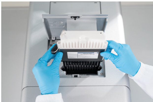
Figure 9. Installation of QIAxcel Gel Cartridge.
