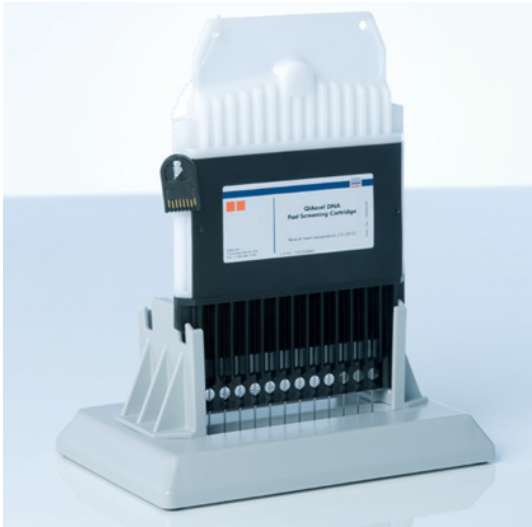
Figure 7. Incubating in the QX Cartridge Stand.
