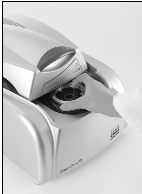
Figure 3. Transferring the samples to the Rotor-Gene Q. After sample preparation and assay setup, the reactions are loaded in the 72 Well or 72 Disc Rotor of the Rotor-Gene Q for real-time PCR analysis.
