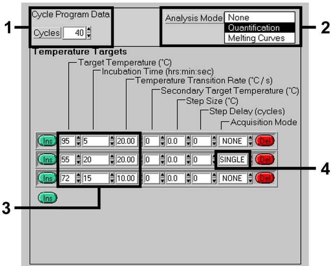
Fig. 5: Amplification of the DNA.
