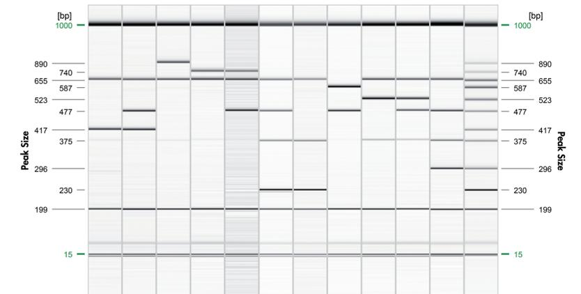
QIAxcel analysis of 11 isolates tested with 11-gene mPCR. The mPCR included the major *E. coli* virulence genes, *stx1*, *stx2*, *eae*, and *ehxA*, and *E. coli* O-antigens from O26, O45, O103, O111, O121, O145, and O157 serogroups. Lane A12 was amplified from a DNA mixture of 7 O-types, and serves as a size marker.
