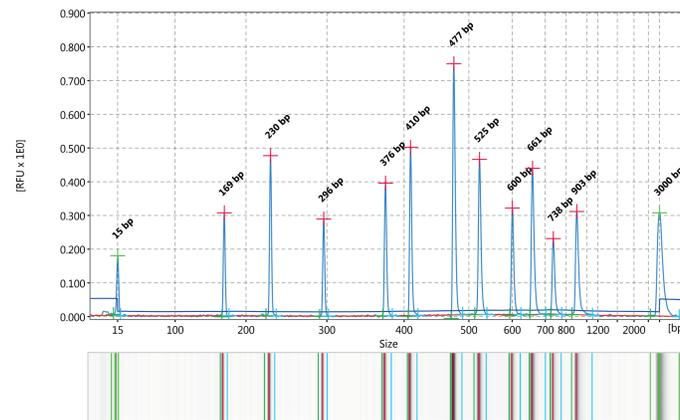
Electropherogram of the control sample. All 11 amplicons used for identification were clearly visible and well separated.
