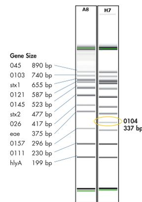
QIAxcel generated gel image showing the separation of products from a 12-gene mPCR.
