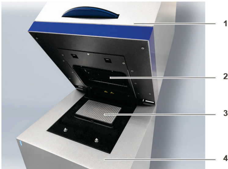
Figure 1. Layout of the QIAquant 384. 1: Upper part with fluorescence spectrometer, 2: heated lid, 3: sample block, and 4: thermal cycler.
