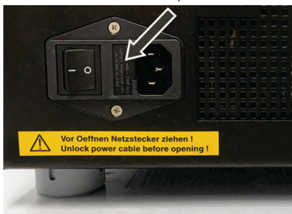
Figure 8. Fuse holder on the rear of the device.
