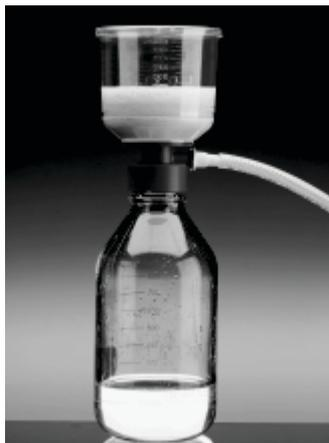
**Figure 3.** The vacuum-operated QIAfilter Mega-Giga Cartridge in use. Note that the bottle is not included in kits.
