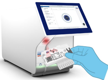
Figure 12. Scanning QIAstat-Dx Meningitis/Encephalitis Panel Cartridge bar code.
