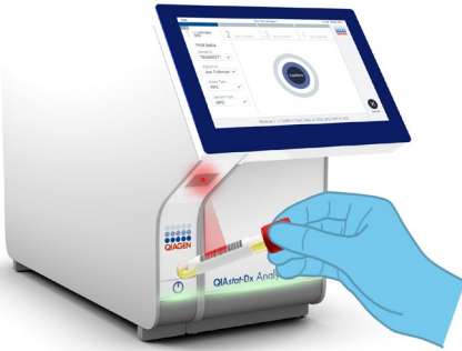
Figure 11. Scanning sample ID bar code.
