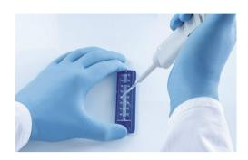
Figure 4. Loading samples into the slide wells.
