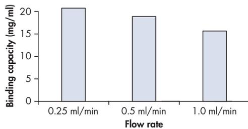
**Figure 2. High-capacity dynamic binding of Glutathione HiCap Matrix.** Yield of GST-tagged protein achieved using the Glutathione HiCap Cartridge (1 ml) depends on flow rates. Dynamic binding capacity is approx. 20 mg/ml; recommended flow rate for the 1 ml cartridge: 0.25–1 ml/min.
