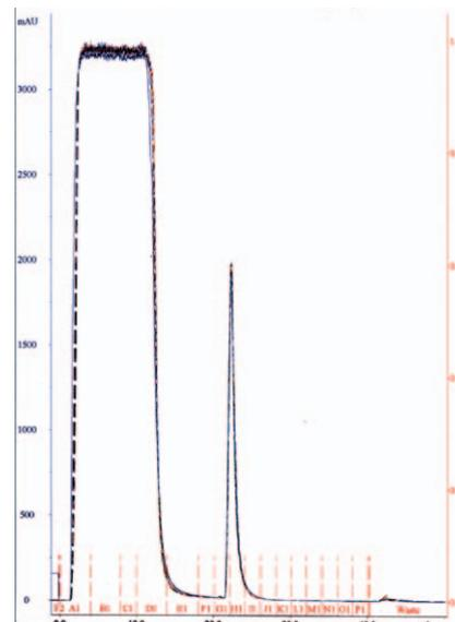
**Figure 4. Highly reproducible purification with Ni-NTA.** His-tagged pGAPase was purified in 10 sequential purification procedures using FPLC. Column load was 10 ml aliquots of cleared *E. coli* cell lysate containing 30 mg spiked protein. Between purification runs, the column was cleaned in situ using 0.5 M NaOH. Overlay of 10 chromatograms is shown.
