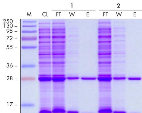
**Figure 1. Purification of highly-pure GST-tagged protein using Glutathione HiCap Matrix.** GST-tagged protein (19 mg) was purified using Glutathione HiCap Matrix and analyzed by SDS-PAGE. 1-2: Two purification procedures with same sample source; CL: Cleared lysate; FT Flow-through; W: Wash; E: Eluate fractions; M: Markers.
