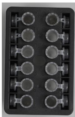
Lids of sample tubes must be securely placed into the slots at the edge of the shaker rack
