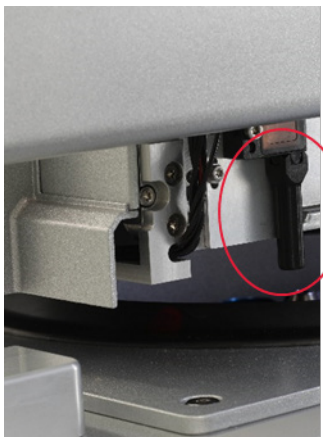
Black beam columnator (see red circle) of the ultrasonic sensor
