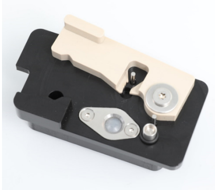
O-Ring tool with prepared new O-Ring
