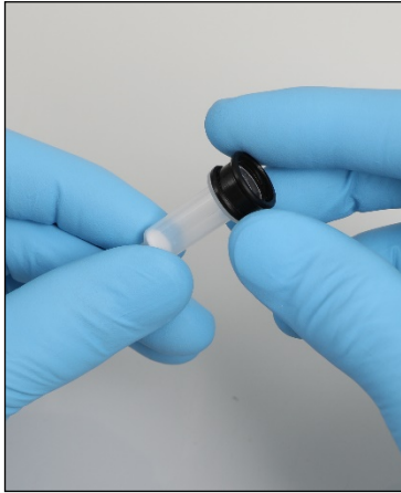
Mounting a spin column adapter ring.
