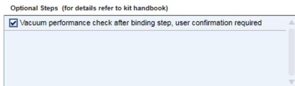
If the vacuum performance check step is checked, the instrument will pause after the binding step. The user can then look to see whether all liquid has passed through the membranes and decide whether to switch on the vacuum again (**Re-do vacuum**) or to continue (**Proceed**).
