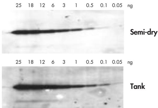
**Figure 7.** The indicated amounts of purified 6xHis-tagged DHFR mixed with crude extract from HeLa cells (8  $\mu$ g total protein) were applied to an SDS-polyacrylamide gel. Western blots were prepared in an electrophoretic transfer apparatus according to the method indicated. 6xHis-tagged protein was detected with Penta-His Antibody diluted 1/2000 followed by HRP-conjugated rabbit anti-mouse IgG and ECL™ detection system.
