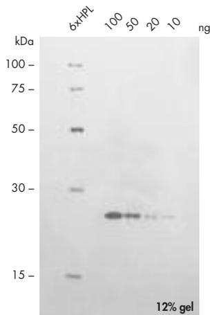
**Figure 11.** The indicated amounts of purified 6xHis-tagged DHFR mixed with crude extract from *E. coli* cells (8 µg total protein per lane) were applied to a 12% SDS-polyacrylamide gel. After electrophoresis and western transfer, 6xHis-tagged proteins were detected with Penta-His Antibody followed by chromogenic detection with AP-conjugated rabbit anti-mouse IgG and NBT/BCIP detection reagent. 6xHPL: 6xHis Protein Ladder (2.5 µl).
