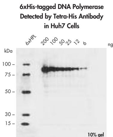
**Figure 4.** The indicated amounts of purified 6xHis-tagged DNA polymerase mixed with crude extract from Huh7 cells (5 µg total protein per lane) were applied to a 10% SDS-polyacrylamide gel. After electrophoresis and western transfer, 6xHis-tagged proteins were detected with Tetra·His Antibody followed by chemiluminescent detection with AP-conjugated rabbit anti-mouse IgG and CDP-Star™ detection reagent. **6xHPL:** 6xHis Protein Ladder (2.5 µl).
