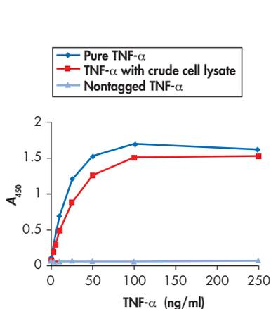
**Figure 16.** Purified 6xHis-tagged protein was bound to Ni-NTA HisSorb Strips for 1 h at room temperature, either alone or mixed with crude cell lysate at 5 mg/ml. As a control, nontagged protein was also applied. Bound TNF-α was determined using anti-TNF-α-peroxidase conjugate for 1 h at room temperature followed by determination of enzyme activity using OPD as substrate.
