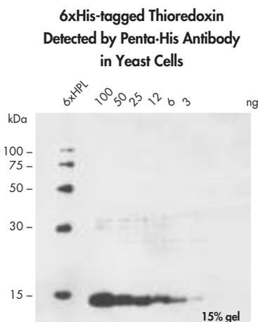
**Figure 5.** The indicated amounts of purified 6xHis-tagged thioredoxin mixed with crude extract from yeast cells (5 µg total protein per lane) were applied to a 15% SDS-polyacrylamide gel. After electrophoresis and western transfer, 6xHis-tagged proteins were detected with Penta·His Antibody followed by chemiluminescent detection with HRP-conjugated rabbit anti-mouse IgG and ECL™ detection reagent. **6xHPL:** 6xHis Protein Ladder (2.5 µl).
