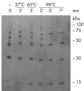
**Figure 9.** Effect of insufficient heating. The 6xHis Protein Ladder was dissolved as described above and heated at different temperatures for the different times shown. After electrophoresis and western transfer, 6xHis-tagged proteins were detected using Penta-His Antibody followed by AP-conjugated anti-mouse antibody and chromogenic substrate (BCIP/NBT).
