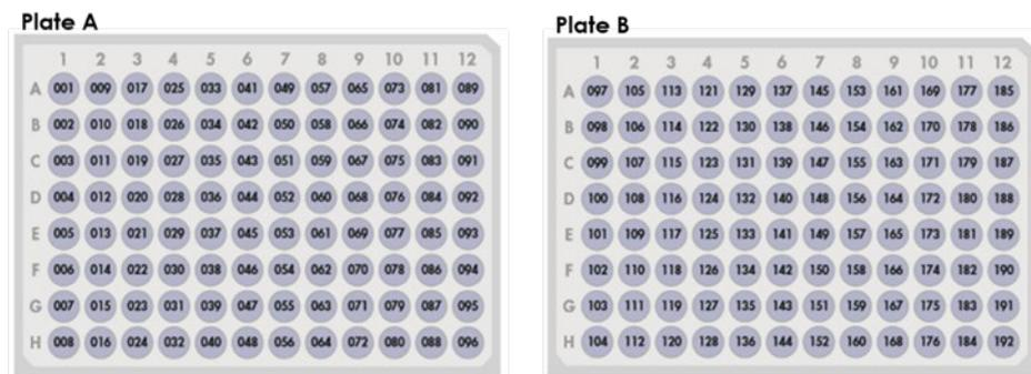
**Figure 5. Layout of the pierceable QIAseq 96-Unique Dual Index Set Adapter Plates.** QIAseq 96-Unique Dual Index Set A (96) layout (SQDIB001- SQDIB096) and QIAseq 96-Unique Dual Index Set B (96) layout (SQDIB097- SQDIB192).
