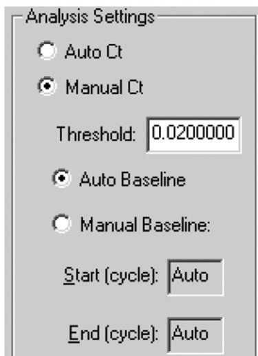
Figure 1. Adjusting the analysis settings for the Applied Biosystems 7500. Select “Manual Ct” and “Auto Baseline”.
