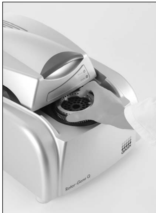
Figure 6. Transferring the samples to the Rotor-Gene Q. After sample preparation and assay setup, the reactions are loaded in the 72-Well Rotor of the Rotor-Gene Q for real-time PCR analysis.
