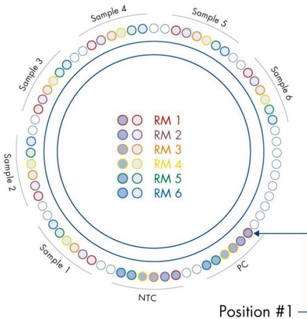
**Figure 5. Plate and rotor setup for an experiment with the PIK3CA RGQ PCR Kit.**
