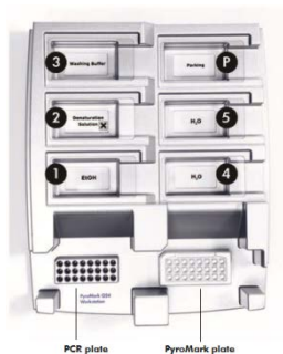
Figure 1. Placement of PCR plate and PyroMark Q24 plate on the vacuum workstation.
