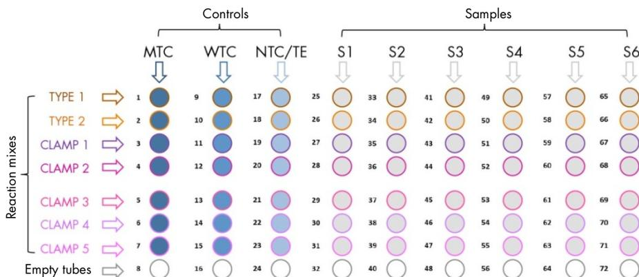
**Figure 4. Loading block setup for an experiment with the *ipsogen* CALR RGQ PCR Kit.**
