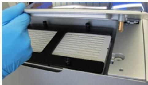
5. Unscrew the four thumb screws. See schematic in the step-by-step wizard.
