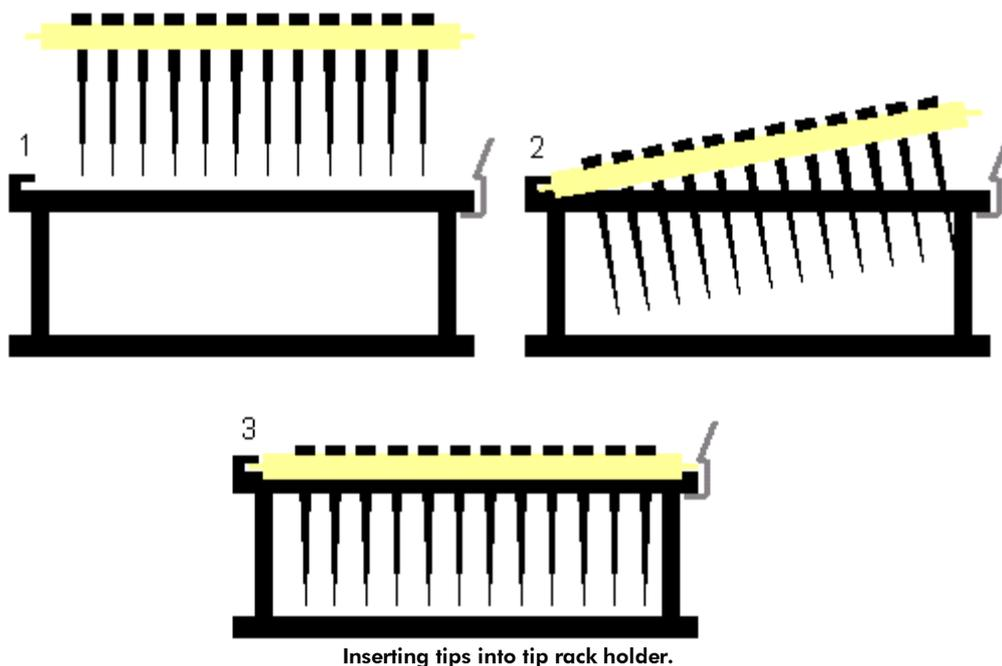
**Note:** Sometimes, the tip rack holder may not fit perfectly into the worktable position. In this case, check that the tip rack holder is shifted towards the upper left corner of the worktable position and is aligned with the corner, to ensure calibration and run accuracy.
