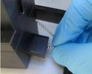
2. Remove the tip ejector by carefully pulling the tip chute upwards.
