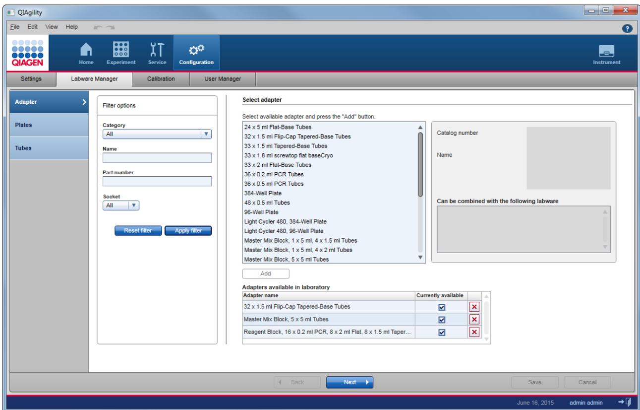
This screen contains a step marker with three steps (**Adapter**, **Plates**, **Tubes**) on the left. The software distinguishes between the different labware types, because they must be treated differently during worktable planning:
