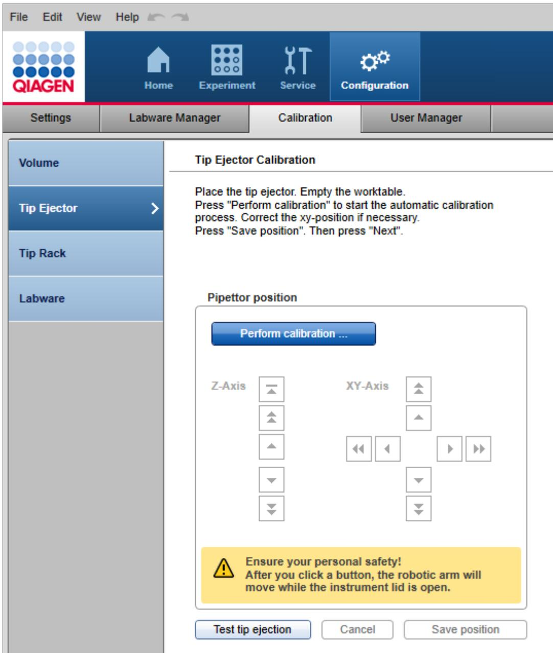
The lid interlock is disabled during calibration. The robotic arm will move during calibration when the lid is raised.
