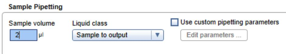
4. The liquid class used for sample transfer is predefined by default.
