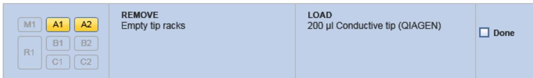
Instruction to remove empty tip racks from worktable positions A1 and A2 and to load full 200 µl tip racks, instead.
