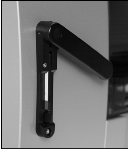
Figure 8. EZ1 Card completely inserted into EZ1 Card slot.
