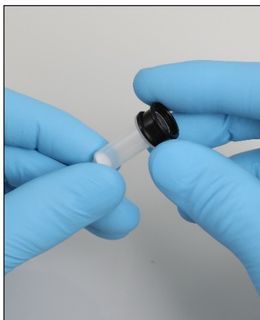
Montering af en spin-kolannes adapterring.
