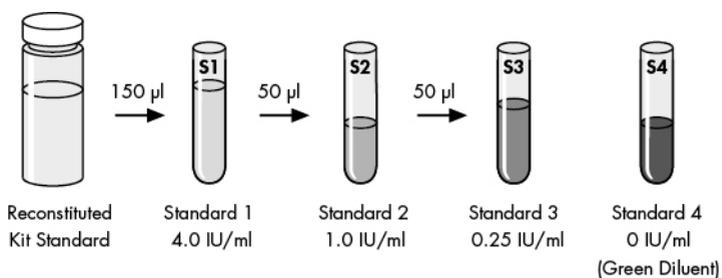
**Figure 4. Preparation of standard curve dilution series.**
